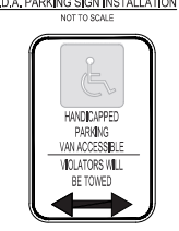
A.D.A. PARKING SIGN INSTALLATION NOT TO SCALE
